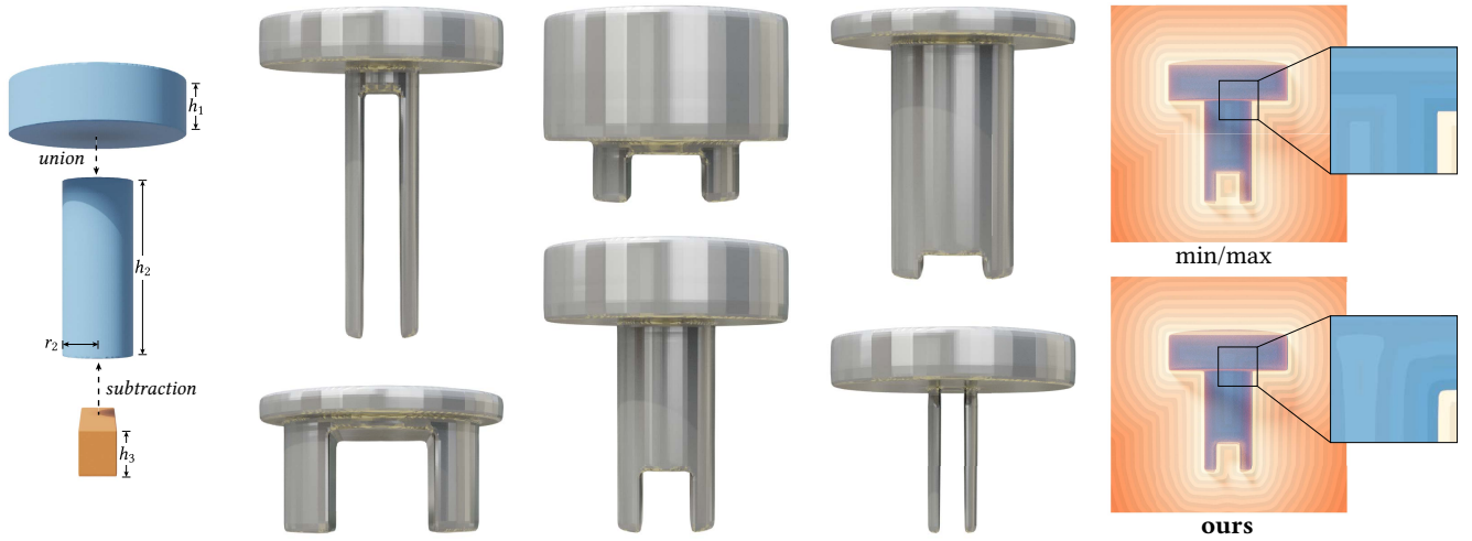
Figure 16: Given a family of pin shapes controlled by (h_1, h_2, r_2, h_3) (left), we use our method to train a parametric neural implicit to represent the exact SDFs of all CSG operations in this family (middle). On the right, we compare the implicit function of a particular instance within this pin family computed naïvely with min and max operations (top right) and as a neural SDF with our regularization applied during training (bottom right).
